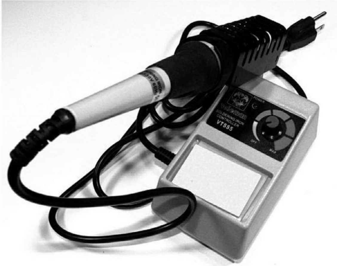
Figure A.19 : Station de soudage.
