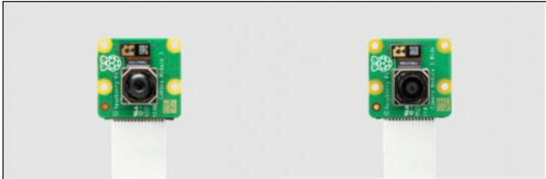
Camera Module 3 (left) and Camera Module 3 Wide (right)
