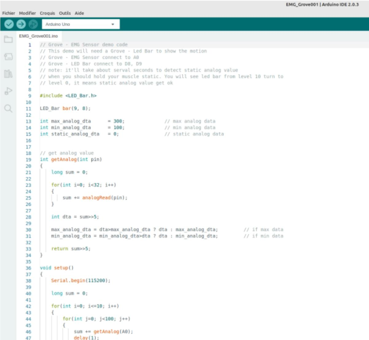
The screenshot shows the Arduino IDE interface with the title bar "EMG\_Grove001 | Arduino IDE 2.0.3". The menu bar includes Fichier, Modifier, Croquis, Outils, Aide, and an Arduino Uno board selection. The code editor displays "EMG\_Grove001.ino" with the following content:
