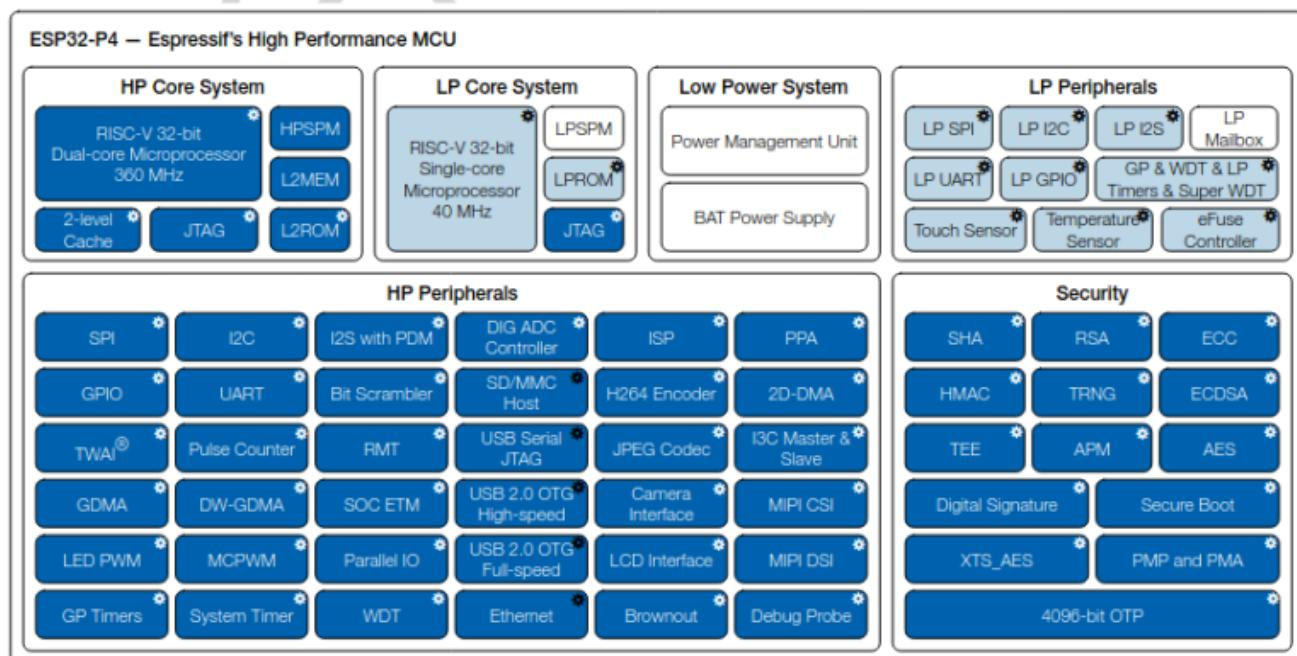
ESP32-P4 Functional Block Diagram
