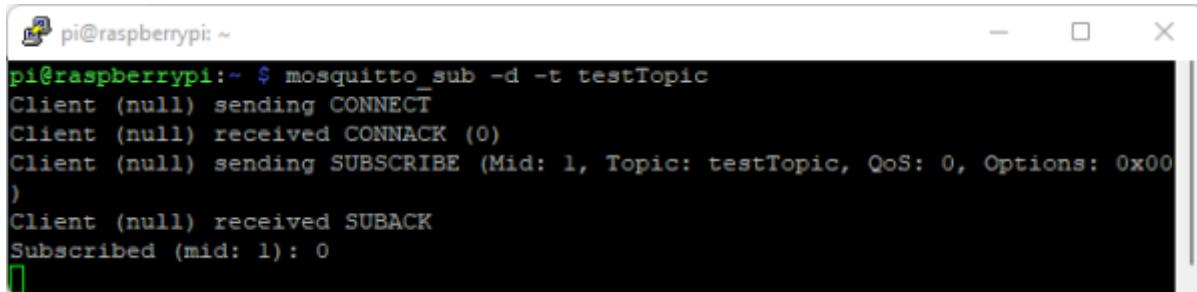
A screenshot of a terminal window titled 'pi@raspberrypi: ~'. The window shows the command 'mosquitto\_sub -d -t testTopic' being run. The output of the command is displayed, showing the client connecting, subscribing to the 'testTopic', and receiving a SUBACK message. The terminal window has a standard Linux-style interface with a title bar and scroll bars.
