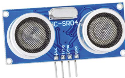
Figure 6.30 The HC-SR04 ultrasonic distance sensor module
