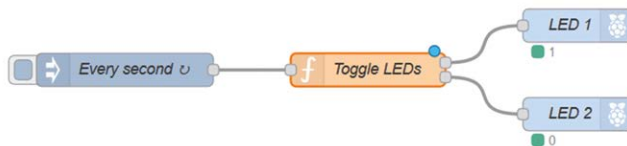
Figure 5.20 Flow program of the project
