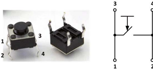
Figure 5.50 Small button and its connection diagram
