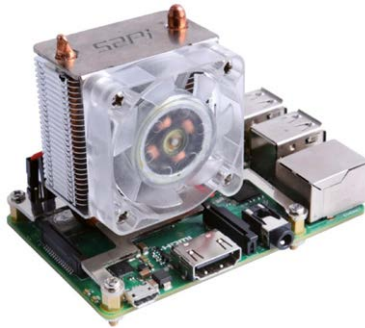
Figure 1.3 Raspberry Pi 4 CPU fan ( www.seeedstudio.com )
